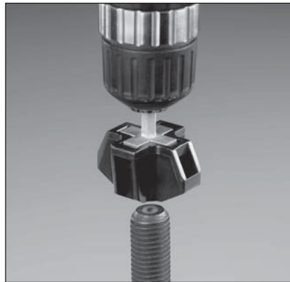
During installation, the custom Stud Mount drill bit ejects itself from mounting base, ensuring proper torque and preventing cracking or breaking of the mount from being overtightened.
