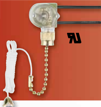
70290 Replacement Canopy Light Switch With Brass Pull Chain 2' Braided Cord 6" Wire Leads Height - 1 1/4" Fits 3/8" Hole
