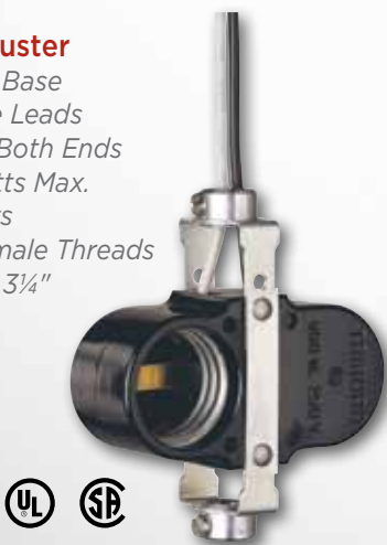
* 22259 Twin Cluster Socket with Male Threads on Each End 6" Wire Leads 18 Gauge, 105° Leads 660 Watts Max. 250 Volts 1/8-IP Nipple Height - 4 1/2"
