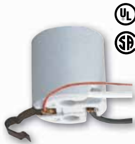
* 22372 Socket Medium Base 9" Wire Leads Fits 3/8" x 1/4" Hole 18 Gauge, 105° Leads 660 Watts Max., 250 Volts Height - 2"
