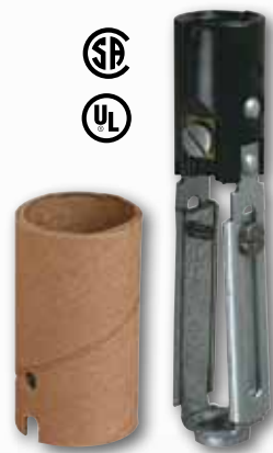
* 22127 70402 (Carded 2-Pack) Adjustable Keyless Socket Candelabra Base 1/8-IP Threaded Hickey 75 Watts Max., 125 Volts Height Adjustable from 3 1/4" - 4 3/4"
