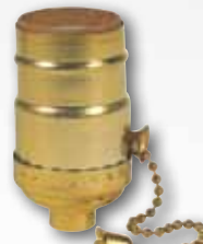
70411 - On/Off 250 Watts Max., 250 Volts 70431 - 3-Way 250 Watts Max., 250 Volts Pull Chain Socket Brass Finish Medium Base Tapped 1/8-IP
