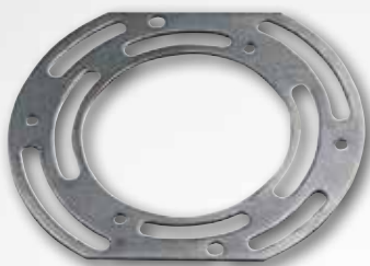
* 21038 Circular Crossbar 4 Holes Tapped 8-32 2 3 / 4 " Center to Center 3 1 / 2 " Center to Center 45 lb. Load Rating
