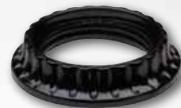
70435 Phenolic Shade Ring For Medium Base Sockets Outside Diameter - 2 3 / 16 " Inside Diameter - 1 1 / 8 "
