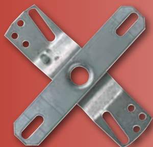
* 21006 70114 Offset Crossbar 4" Long 8-32 Tapped Holes Green Ground Screw 35 lb. Load Rating
