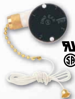
77021 - Single Capacitor, 4-Wire Unit 3-Speed Fan Switch With Polished Brass Pull Chain, 2' Braided Cord 3A, 250 VAC 6A, 125 VAC
