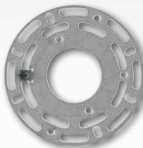
* 21031 Universal Crossbar 6 Holes Tapped 8-32 1 1 / 2 " Center Hole 3 7 / 8 " 2 1 / 8 " Center to Center 2 3 / 4 " Center to Center 3 3 / 8 " Center to Center Green Ground Screw 35 lb. Load Rating
