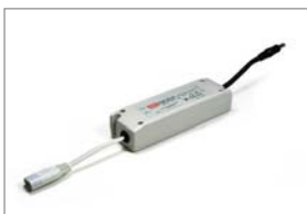
Hardwired Class II Electronic Driver NAPK-530HW/12 12V, 30W NAPK-560HW/12 12V, 60W NAPK-530HW 24V, 30W NAPK-560HW 24V, 60W Requires NUSP-JBox for hard wiring or NRA-6035 for direct plug-in Non-dimmable
