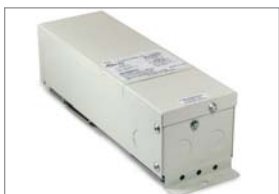
Class II Hardwire Electronic Driver with Integral Regulator for Constant Current and Voltage NATL-5060HW 24V, 60W NATL-5100HW 24V, 100W Includes Hardwire Box and 10' Power Line Connector
