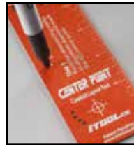
Step 4: Mark the center of the hole.
