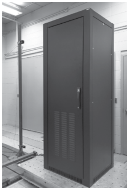
Enclosure mounted on shaker table
