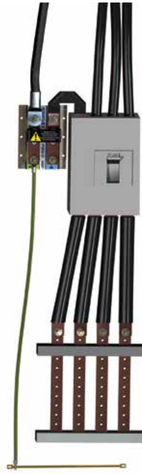
Dedicated TN-S Power Supply
