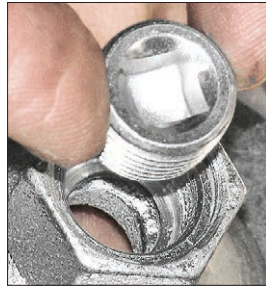
NO-SLIP square-head driver to tighten
