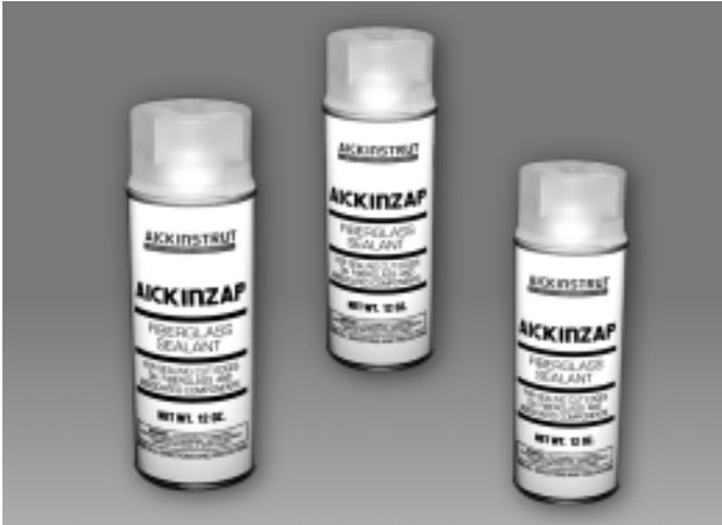
Aickinzap is an acrylic spray that provides a corrosion resistant coating when applied to cut sections of Aickinstrut. Aickinzap is supplied in a 12 oz. can and is recommended for use as a sealant for Aickinstrut polyester and vinyl ester materials after cutting or drilling. Aickinzap is the quickest, most convenient method for sealing after fabrication.
