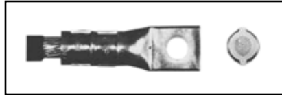
Circumferential compression is solid and symmetrical. No sharp flash.
