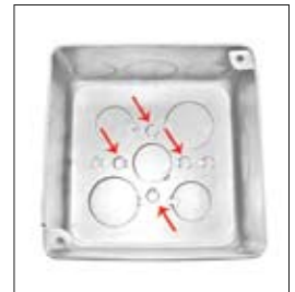
52171-SVT IN USE Patented air tight slugs easily pop out with screw driver for 1/4"-20 threaded rod. No on-site drilling required!
