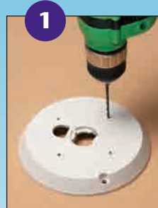
1 Use your camera base as a template and drill holes.
