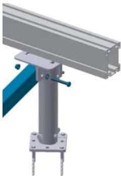
Install the SunBeam Rail on the Pipe Caps. See SunBeam are on page 31.
