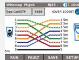
Crystal clear graphical interpretation of results like Wiremap through large 3 1/2" QVGA colour display
