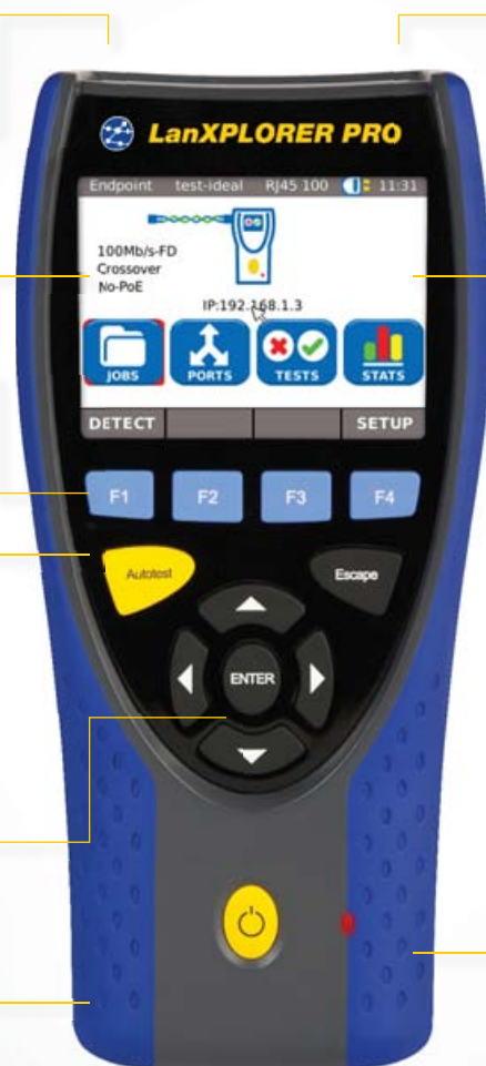
Touchscreen menu navigation allows tests to be completed within three steps
