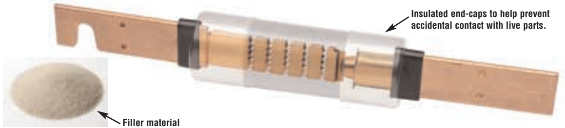
Figure 6. This is the LPS-RK100SP, a 100A, 600V LOW-PEAK®, Class RK1, Dual-Element Fuse that has excellent time-delay, excellent current-limitation and a 300,000A interrupting rating. Artistic liberty is taken to illustrate the internal portion of this fuse. The real fuse has a non-transparent tube and special small granular, arc-quenching material completely filling the internal space.
