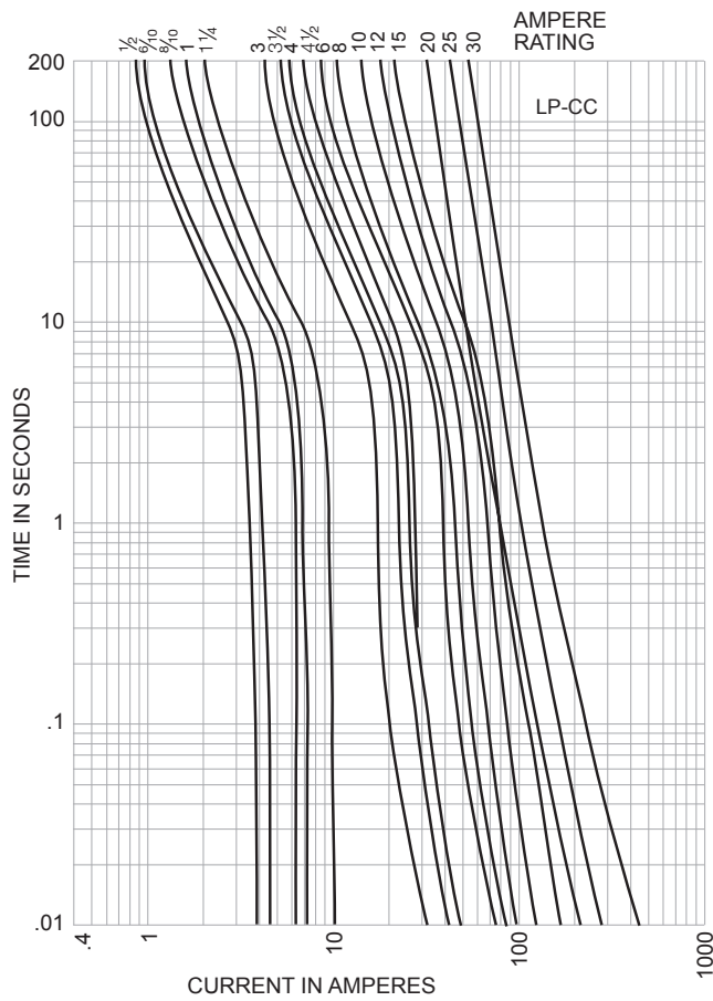
Time-Current Characteristic Curves—Average Melt
