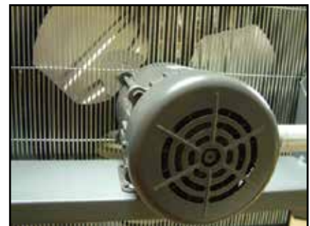
Hazardous Location Rated Motor
