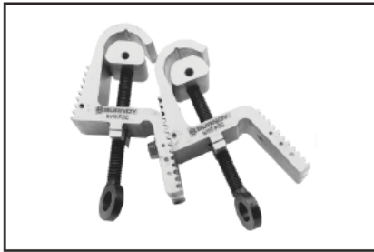
TYPE WHSPBC WEJTAP™ hotstick dual cable clamp used to hold run and tap conductors in position during hotline installation. Universal for all applications from #8-1272 ACSR.
