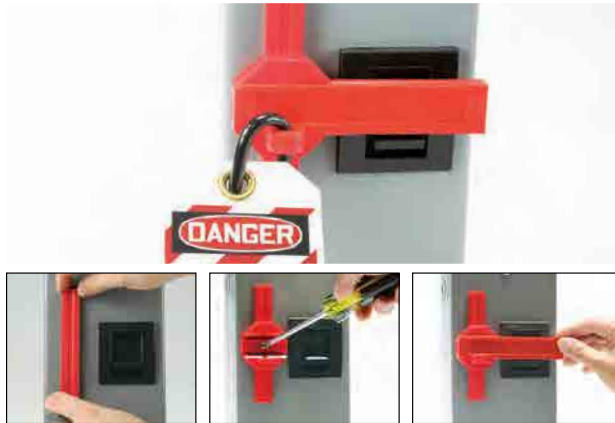
Position Mounting Rail Secure Slide Set Slide Stop Bar into position over breaker
