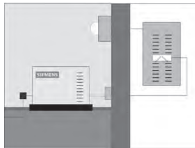
Generator Ready Load Center with Automatic Standby generator installation
