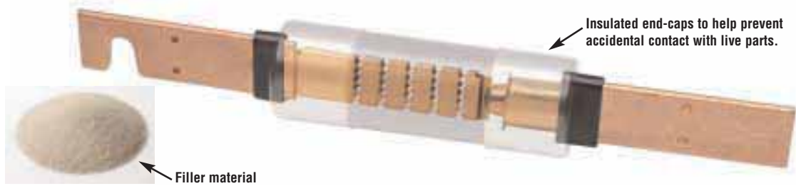
Figure 6. This is the LPS-RK100SP, a 100A, 600V LOW-PEAK®, Class RK1, Dual-Element Fuse that has excellent time-delay, excellent current-limitation and a 300,000A interrupting rating. Artistic liberty is taken to illustrate the internal portion of this fuse. The real fuse has a non-transparent tube and special small granular, arc-quenching material completely filling the internal space.
