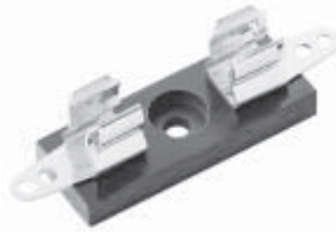
4520 and 4393 Single Pole Fuseblock for 1/4" x 1" Fuses Bakelite base; Width 1/2" (12.7mm). Spring-bronze, bright tin-lead plated clips. Rated 30A, 250V.
