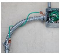
Use the 407-DC2G grounding connector in conjunction with the 281-DCG transition fitting to connect and bond the flexible metal conduit system to EMT.
