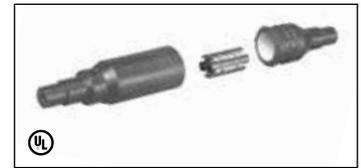
The uniquely designed interference fit cover enables direct burial of UF Cable to be a quick and reliable process. The kit includes a mechanical connector, silicone lubricant and the interference fit covers. Accommodates 14 AWG to 8 AWG wire sizes.
