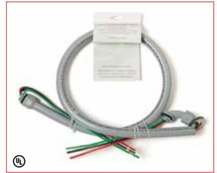
Designed to save the contractor installation time and labor, our Air Conditioner Whips are typically used to connect the Central Air Conditioner Compressor to the AC disconnect box. Air Conditioner Whips include one (1) Straight and one (1) 90° Connector. Three (3) Conductors are included in 1/2" or 3/4" Non-Metallic Liquid Tight Conduit using either 8 or 10 AWG THHN Conductors.
