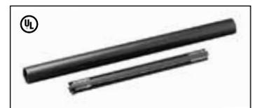
Simplify UF Cable repairs after a trencher or backhoe has damaged or destroyed a 7" to 10" section of UF Cable. Utilize our Thick Wall Heat Shrink Tubing with sealant to make a quick and reliable repair. Eliminates epoxies, tapes or separate mastics and creates a waterproof splice. The kit includes one (1) 4-position 11.5" connector and one (1) piece of heat shrink tubing. Designed to splice and insulate 14 AWG to 8 AWG UF Cable.
