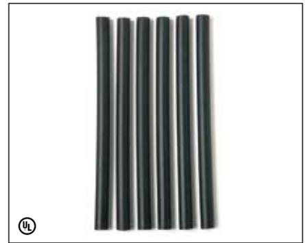
Thick Wall Heat Shrink Tubing (HST) is used to dielectrically insulate and encapsulate electrical connections. The HST internal coating has an adhesive and sealant that melts when the tubing is heated to provide a moisture and soil resistant seal. The standard color is black.
