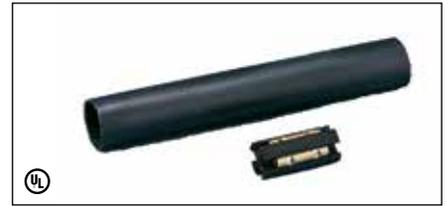
The UF Cable Splice Kit includes one (1) 4-position mechanical connector and one (1) piece of heat shrink tubing to splice and insulate 14 AWG to 8 AWG UF Cable.
