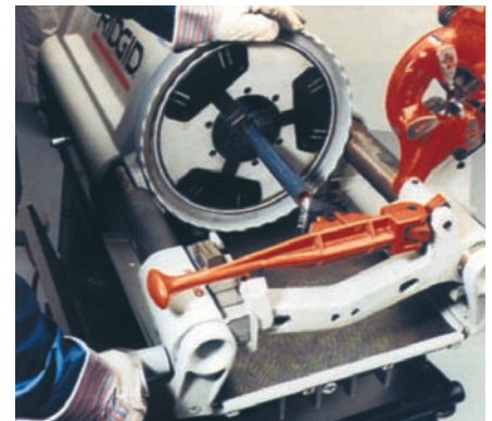
Use a reamer to remove rough edges.
