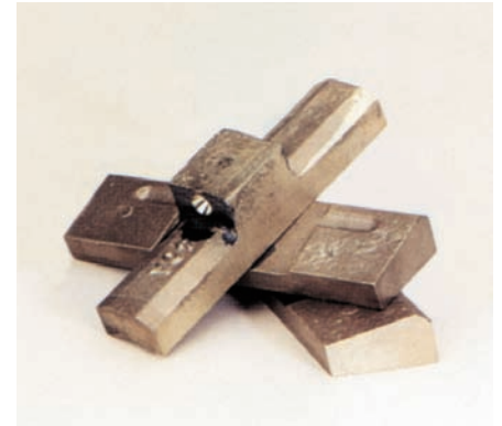
Jaws 3 was designed to protect Plasti-Bond REDH 2 OT conduit from damage by vise jaws during conduit bending.
