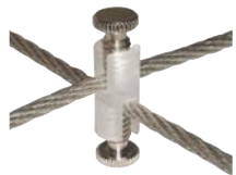
Cross Isolators Pair (CA-338) Secures and electrically isolates Cables crossing at 90°. Isolators constructed from clear Lexan™. Bolt heads available in aluminum, Polished nickel or Rubbed bronze.
