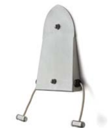
Power plate (CA-508) Covers standard single gang box and delivers low voltage power from remote transformer to the Cable system. Single feed only. 36" power cable leads and power bolts provided. Typically wall mounted.
