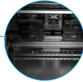
Four-fan unit and vent holes provide optimum ventilation
