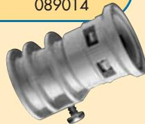
Both styles of stub down fittings are designed for direct connection to ENT on the horizontal by means of our patented six locking tab concrete-tight Kwikon connection. The flanged base of the threaded 90° stub down offers contractors a NPSC threaded hub connection on the vertical – at the exit point of the slab, allowing for the direct transition to other raceway products.
