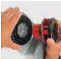
Inserting the die heads
