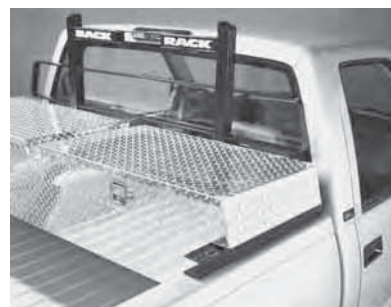
Special Toolbox Brackets accommodate any crossbed toolbox.
