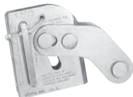
Model GVV655 Stainless steel rope grab for use with 5/16" diameter stainless steel wire rope. Can be attached, detached, and positioned at any point on the vertical lifeline.
