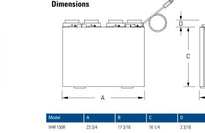
Dimensional information is in inches. Clearance of 17" in front of the unit is recommended for removal of core. The unit features a three foot plug-in power cord with 3-prong plug.
