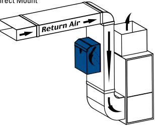
Furnace fan should operate continuously when HEPA unit is on and running. The return side of the furnace is the recommended location for the HEPA to connect to. The supply side is normally avoided due to the higher static pressure.
