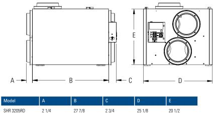
Dimensional information is in inches, Clearance of 12" in front of the unit is recommended for removal of core
