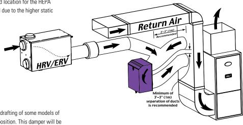
A power damper is recommended to prevent backdrafting of some models of air to air exchangers, when in the off or standby position. This damper will be installed between the HRV/ERV and the HEPA unit.
