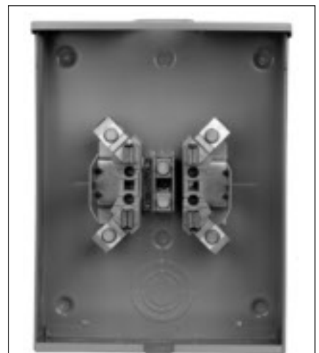
SUAT417-XG 4-Jaw 1Ø 3W 200 Amp Residential - No Bypass
