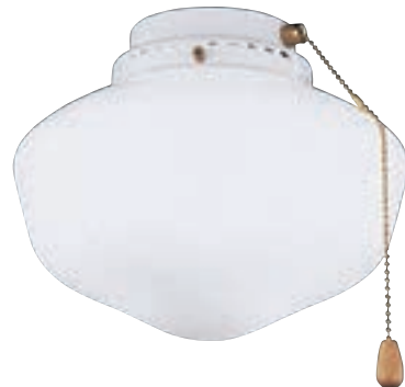
CFSLK1 SCHOOLHOUSE SINGLE LIGHT FIXTURE (6.33" H X 8.5" W) Available in WW. One 23-watt medium base compact fluorescent bulb (included). Rated for one 100-watt incandescent.
