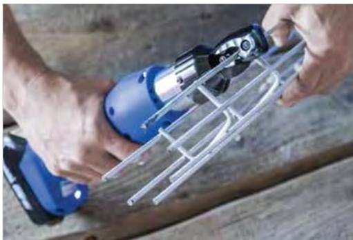
Small head size permits cuts close to welds
