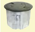
CRFB SERIES<br>CRFB4 | Surface                 | Wood, Raised                  | Round       | Triple             | 4 gangs      | Die-Cast Aluminum | 2 1/4" [57mm]              | 1/2", 3/4", 1", 1 1/4" & 2" Trade Size | Carpet, Tile                                    | Die-Cast Aluminum                    | CRFBCTC, CRFBTTC, Evolution Series 8AT |                                                |  |
