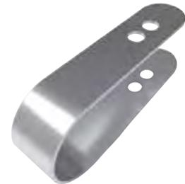
The RS1™ rod stiffener is used with 1" Schedule 40 or Schedule 10 steel pipe and 3/8", 1/2" and 5/8" hanger rod. It snaps over the pipe and rod, and connects easily with a provided bolt and lock nut.
