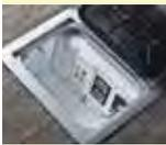
EFB45S                 | Recessed                | Concrete, Wood, Raised Floors | Rectangular | Triple             | 4-5 Gangs    | Steel             | 3 1/2" [89mm]              | 3/4" - 2" Trade Size                   | Tile, Carpet, Wood, Terrazzo, Polished Concrete | Die-Cast Aluminum                    | EFB45CT, EFB45BT, EFB45T, EFB45CT      | Removable Modules, Standard Size Device Plates |  |
