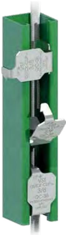
The Quick Clip™ is the fastest, easiest-to-use rod stiffener on the market. For use with 1-5/8" x 1-5/8" 12-gage strut and 3/8" or 1/2" hanger rod, the unique design offers effortless one-handed installation in less than 5 seconds — with no tools needed!
