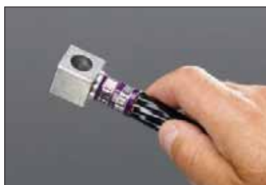
1. Crimp Multi-Tap connectors onto cables.
