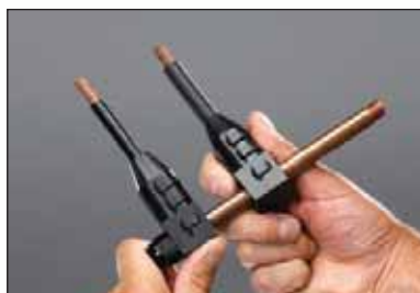
4. Slide connector/insulator assemblies onto rod.
