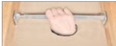
2) Twist out to bite on joists.
