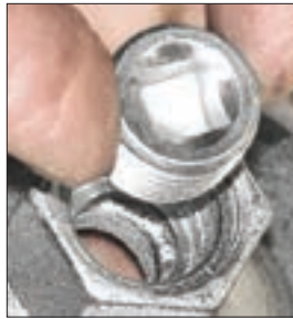
NO-SLIP square-head driver to tighten
