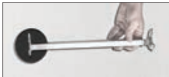
1) Cut hole & insert bracket.
