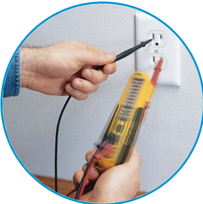
Vibration mode gives a tactile indication of the voltage level.
