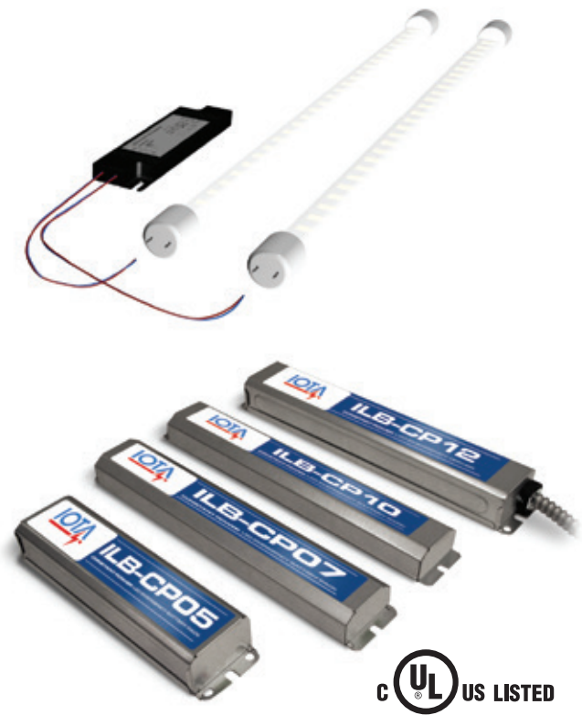
Fig.2 - LED tube lamps with internal drivers do not require a fluorescent ballast. When no external ballast is available to wire the emergency ballast to, an auxiliary supply such as a generator or inverter must be used to provide emergency line power.
