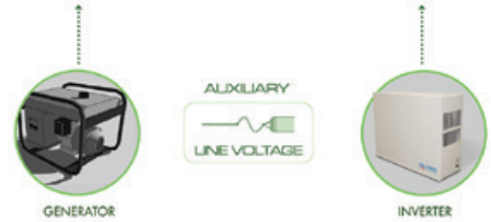
Fig.2 - LED tube lamps with internal drivers do not require a fluorescent ballast. When no external ballast is available to wire the emergency ballast to, an auxiliary supply such as a generator or inverter must be used to provide emergency line power.
