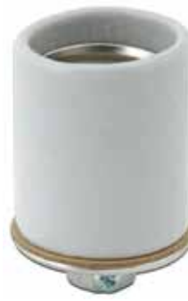
30700 -Porcelain Keyless Socket with metal cap, Tap 1/8 IP Cooper Nickel screw shell, 2" Ht., 30729 -Bulk pack 150per Box. caps, insulators & Sockets
