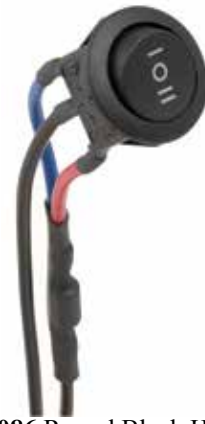
30086 Round Black Hi-Low Rocker Switch. Sequence: Hi-Low Rated: 6A-125V, 3A 250V 6" AWM 105°C Leads Strip 3/4"
