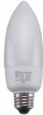
22513 14 Watt (60 Watt) Flame Tip Standard Base 8,000 Hrs. 620 Lumens Ht. 5.61 Dia. 2" 22514 7 Watts (25 Watt) Flame Tip Standard Base 9,000 Hrs. 320 Lumens Ht. 5" Dia. 1.65"
