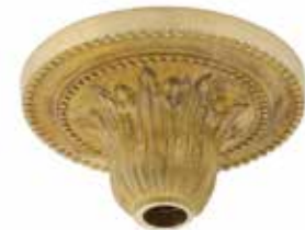
58131 Cast Brass Candle Cup & Plate combination 2 3/4" Dia. Top 1 1/2" Ht. Slip 1/8 IP 7/8" ID
