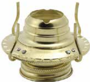
54189 #2 Cut-out Eagle Burner 3" chimney holder. Steel Brass Plated. Fits 54253 or 54356 collars.
