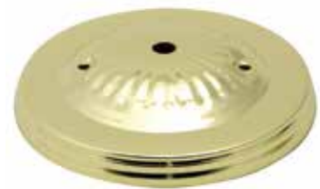
54626 Brass Plated Finish 54625 Antique Finish Steel 5" dia. Canopy, 1 3/8" deep. 1/8 IP center hole, 2 3/4" spaced holes. Ht. 1 1/4"
