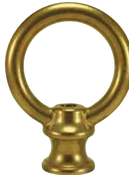
Extra Heavy Giant Loop dia 3 1/2" Ht. 4 1/2" 58304 1/4 IP Tap 58305 3/8 IP Tap 58306 1/2 IP Tap
