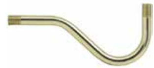
55353 Raw Brass Pin-Up Arm 5 1/2" L x 2 1/4" H 1/8 IP Threaded each end 1/2"
