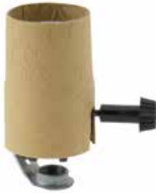
30114 -3-Terminal Turn Knob 1/4" mandrel for wiring top, bottom or both. 4/36 thread hickey is removable use with 30135 . 250W-250V
