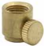
55537 Brass 1/8 F Tap x 1/4 - 27 slip, Side Hole 8/32" Tap Ht. 17/32" Dia 1/2"
