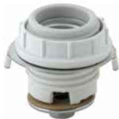
30189 -Porcelain Screw Type Keyless Socket Threaded steel ring, insulated cap 1/8IP, 2" Ht., 2 3/16" ring dia. Comes with Metal & plastic ring. 660W-250V
