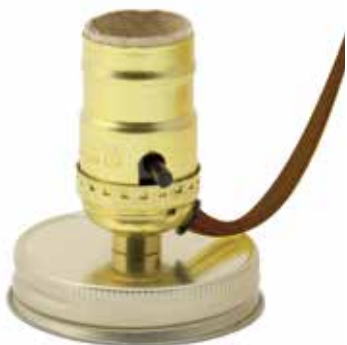
Brass plated mason jar collar kit. Push-thru socket wired. 8' cord Collar 2 3/4" dia. 80321 Brown Cord 80322 Clear Gold Cord 80324 Clear Silver Cord
