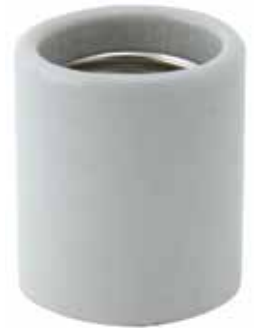
30160 -Porcelain Keyless Socket without cap Leviton Brand. Use with 30706 or 30707 Cap 1 5/8" Ht., 660W-250V
