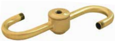
56299 Raw Brass 5 1/2" spread end to end. Cluster is tapped 1/8F x 1/4F. Arm threaded 1/8M. Use 55018 to reduce bottom hole to 1/8 IP
