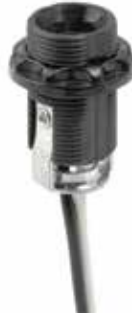
30723 - Threaded Candelabra Socket with ring, 12" leads. Total Ht. 1 1/2" 75W-125V. Use on vanity mirrors
