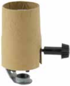
30174 3-Way Socket with 1/4" mandrel. 4/36 thread with hickey 250W-250V
