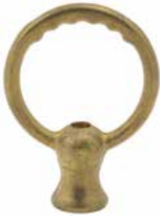
56958 Cast Brass Notched Loop. NOTCHED for chain fixtures to hang straight. Tap 1/8 IP w/wireway Ht. 2 7/8" 2" Width
