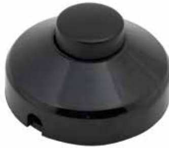
30566 Black Single Pole Lamp Foot Control step on Off/On switch. Unassembled, takes 18/2 SPT-2 and SPT-1 wire. 3A - 125V UR
