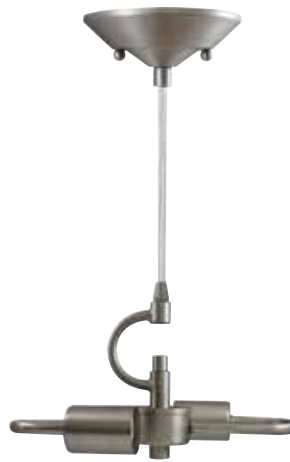
19097 2-Light Shade Adaptor Kit Satin Nickel Finish UL Listed 5" Canopy 7' of Clear SVT/3 Wire
