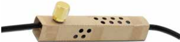
30584 Lamp Tube dimmer halogen 500W - 120VAC Full range w/positive on/off. 19" leads one end, 5" leads other end. Input 110-120V. UL and CSA Listed. 30585 BPL replacement knob.
