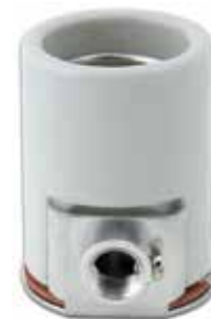
30701 -Medium Base Porcelain Socket with side outlet bushing. 2" Ht. Tapped 1/8 IPS with set screws bushing extends 1/4" beyond edge of socket & centers 7/16" below cap surface with screws terminals .Rated 660W-250V
