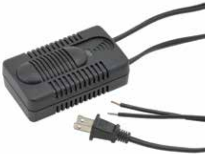
30803 Black Lamp floor dimmer, wired with 9' lead for lamp and 9' cord set with plug. Slide control. 600W max. Tri-level. Input 110-120V. Incandescent and Halogen. UL & CSA Listed.
