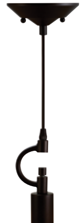
19093 1-Light Shade Adaptor Kit Bronze Finish UL Listed 5" Canopy 7' of Brown SVT/3 Wire
