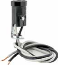
30068 -Bakelite Candelabra Socket 1/2" Hickey from body with 18" leads. 75W-125V
