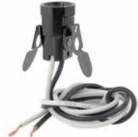
30135 - Bakelite with spring clip Fits 7/8" to 1 1/8" dia, hole base/ 18" leads. 75W-125V
