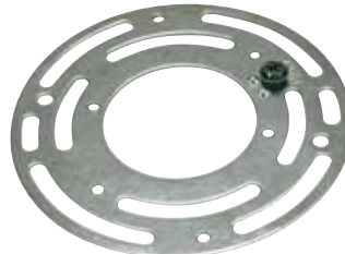
54856 Universal Circle Cross Bar 1 13/16" center hole, 4" outer diameter. 6 holes tapped 8/32 on: 2 1/8" center to center 2 3/4" center to center 3 1/2" center to center
