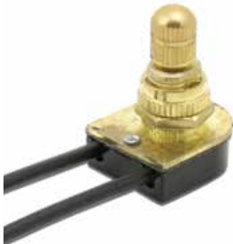
30048 Brass 30049 Nickel Single circuit rotary canopy switch w/6" leads, 3/8" shank. Metal removable knob
