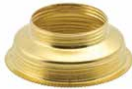
56230 Solid Brass Expander Screws into #1 size collar and fits #2 size burner. 1 7/16" O.D. Has 3/4" I.D.
