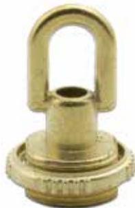
Screw Collar Loop 50108 Antique Brass Finish 50137 Brass Plated 50145 Chrome 50406 White Regular screw collar Loop ring seats 1 1/16" Tapped 1/4 IP F Ht. 1 7/8" Dia 3/4"
