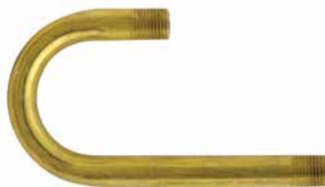
55722 Brass Arm 2" L x 3 1/2" H 1/4" Thread each end
