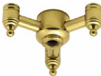
56298 Raw Brass 3 Lite Cluster. 1 1/4" from center to light. 1/8 IP Threaded all openings.
