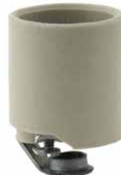
30726 -Porcelain Keyless Socket Tap 1/8 IP, 5/8" Hickey, 1 3/4" Ht. 660W-250V
