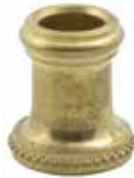
55057 Brass 55421 Burn. & Lacq. Ht. 7/8" Slip 1/8 IP Dia. 13/16"
