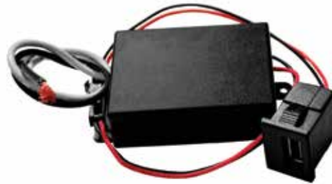
30807 Snap in USB port with transformer kit, class 2 power supply Snap in USB port 13/16" x 21/32" opening. Class 2 100V-240V 50/60HZ input, 5Vdc 200 MA 10W output. Quick connect supply wires. 3" x 2" x 3/4"Ht.
