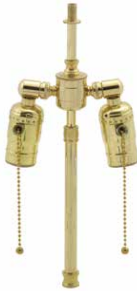
70076 Adjustable Double Cluster Socket Assembly. Unwired each socket is attached to a swivel. Solid brass polished & lacquered except for pipes. 10 1/2" Ht. extends to 13 1/2" Ht. 1/8 IP
