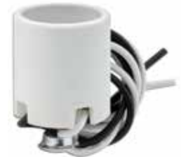
30705 - Medium Base Porcelain Socket with 105° 18" leads, 1/8 IP Hickey 1 7/8" Ht. 660W-250V
