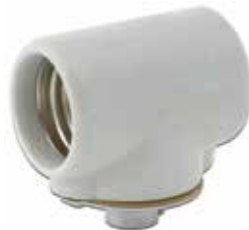
30702 -2" Wide Medium Base Duplex Porcelain Socket. with metal flange cap. Tapped 1/8 IP, with set screw 660W-250V Screw Terminals
