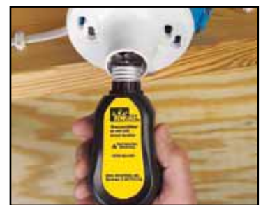
Lighting adapter allows connection to light fixtures.
