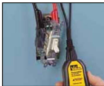
Alligator clip adapter allows connections to exposed wiring.
