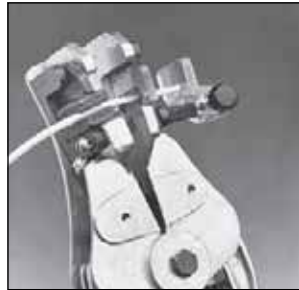
Transparent wire stop provides uniform stripping length.
