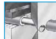
Knife-type stripping blades have form-ground holes which penetrate the insulation like a knife, giving a clean insulation cut.
