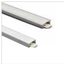
4' Shallow Aluminum Channel NATL-C23A with Wing NATL-C24A Used to mount tape light to various surfaces. Plastic diffuser and end caps included. Field cuttable.
