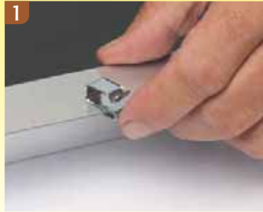
Snap Wire Clip onto sheet metal up to .080" thick.
