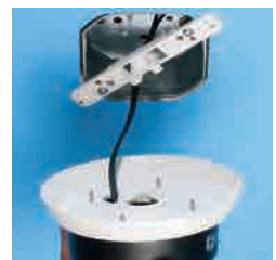
2 Place assembly on bracket. Turn clockwise to lock. Install set screw. Done! Secure camera installation on ceiling or wall.
