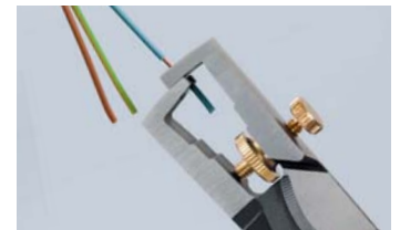
Graduated jaw is a visual orientation aid when stripping wire in standard lengths (11 mm and 16 mm)
