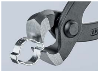
10 98 I220: Using the front press nib
