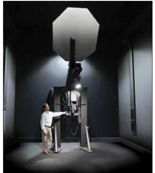
RAB's on-site Goniophotometer provides precision measurement of light output.
