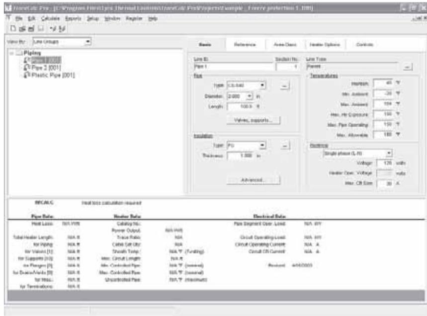
Fig. 1 TraceCalc Pro heat-tracing design software
