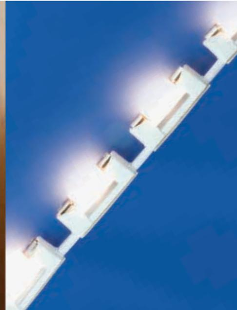
With a bend radius of 2.25" (5.75cm), inside or outside, Xenon Bristrip can evenly illuminate the tightest of curved surfaces. Even 90 degree corners are simple to do. Xenon Bristrip mounts easily with 3M® double sided tape (pre-fixed to the back of each socket) or with simple to use nail clips for added security. The lamp holders have a metal reflector built in which deflects heat away from the mounting surface and reflects light onto the surface being illuminated.
