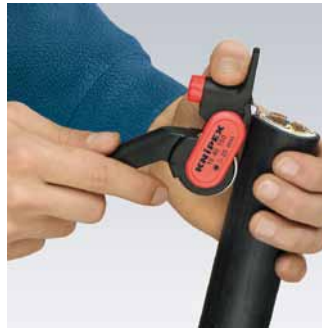
Setting the tool for longitudinal cut
