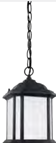
DAMP + ONE LIGHT OUTDOOR SEMI-FLUSH CONVERTIBLE PENDANT L: 6.5" W: 6.5" H: 10.5" Semi-flush H: 9.75" 10' wire pre-laced through 4" chain
