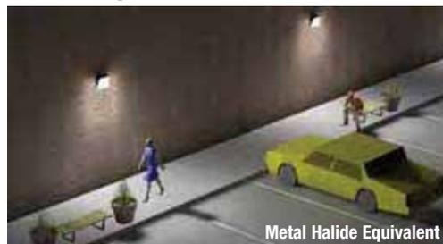
**NOTE:** Typical mounting heights are 8'-12' (10W models) and 8'-25' (20W and 30W models). Simulation rendering using AGI32 Software.
