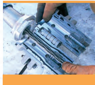
Place the winch line in the main blower body and select the proper venturi.
