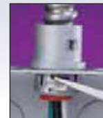
Using a screwdriver, lift the ring and twist off.
