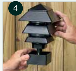
4 Press fit spacer to base of lamp.
