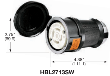
30A 3Ø 250V AC NEMA L15-30R UL/CSA 3 HP
